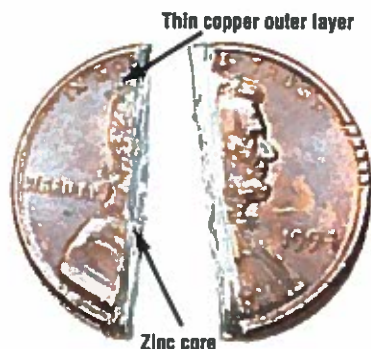
Cross-section showing the structure and composition of a post-1982 penny.
