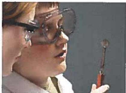
In the morning, remove the mustard. If silver is indeed present, there will be a tell-tale black spot, indicating Ag 2 S.
