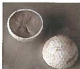
Cryogenic golf ball? Not quite. A golf ball frozen in liquid nitrogen will sometimes split in half on its own. It worked one out of two times for us.
