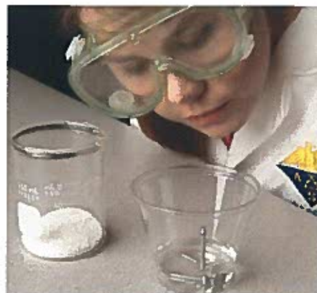
This student investigates the role of salt on the rate of rusting by putting nails in various salt water solutions.
