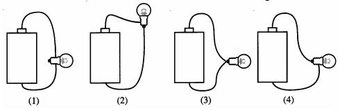
Draw standard circuit diagrams for the four arrangements of battery, bulb and wires shown above.
