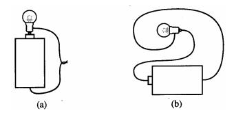
**Question 14.** In which of the following circuits are two wires *required*: only circuit 1, only circuit 2, both circuits, or neither circuit?
