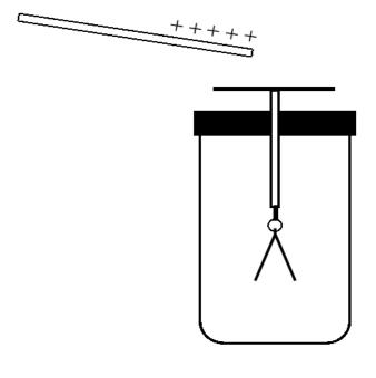
2. The previous experiment illustrates charging by electrostatic induction where a charged body induces an opposite charge in an uncharged body (the electroscope in this case). Explain how this works and why the leaves diverge.
